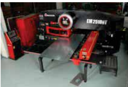
High precision manufacturing facility CNC punch presses most modern electronic turret punch presses with 5 meter table
